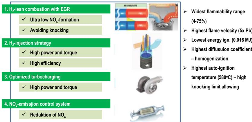
Fig. 17. Hydrogen combustion process in a combustion engine [33]
