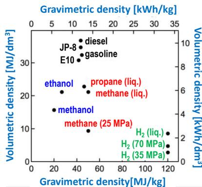
Fig. 7. Energy specifications for liquid and gaseous fuels (including hydrogen) [14]
