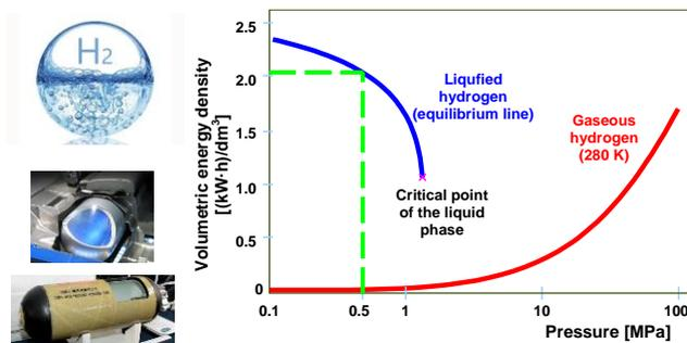
Fig. 5. Physical parameters of liquefied and compressed hydrogen [20]
