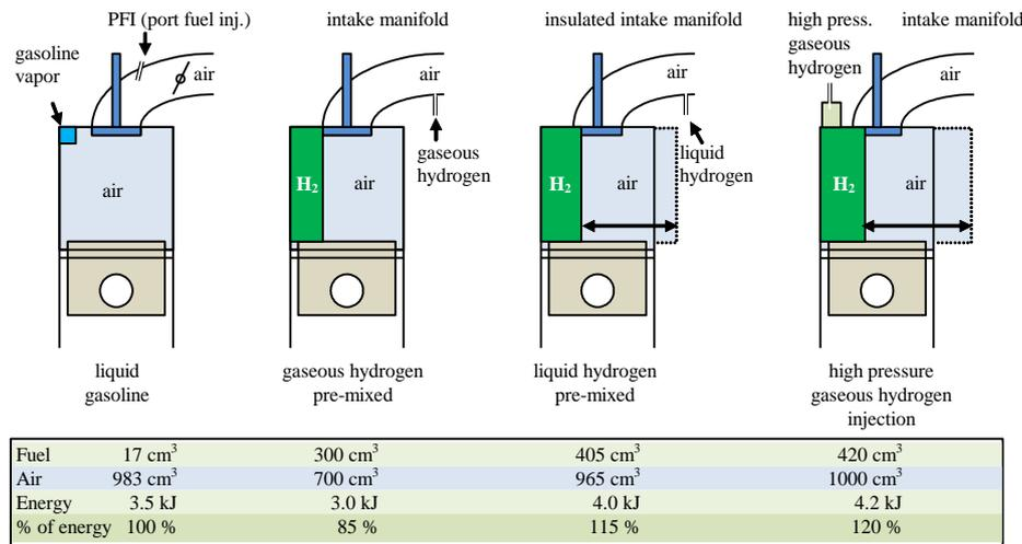
Fig. 13. Hydrogen injection systems for combustion engines [2, 4, 17]
