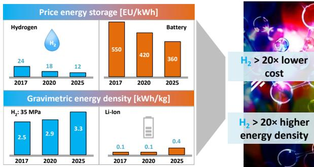
Fig. 1. Energy density of hydrogen and Li-Ion batteries [35]
