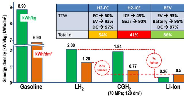
Fig. 11. Hydrogen vs. batteries in vehicle propulsion systems [18]
