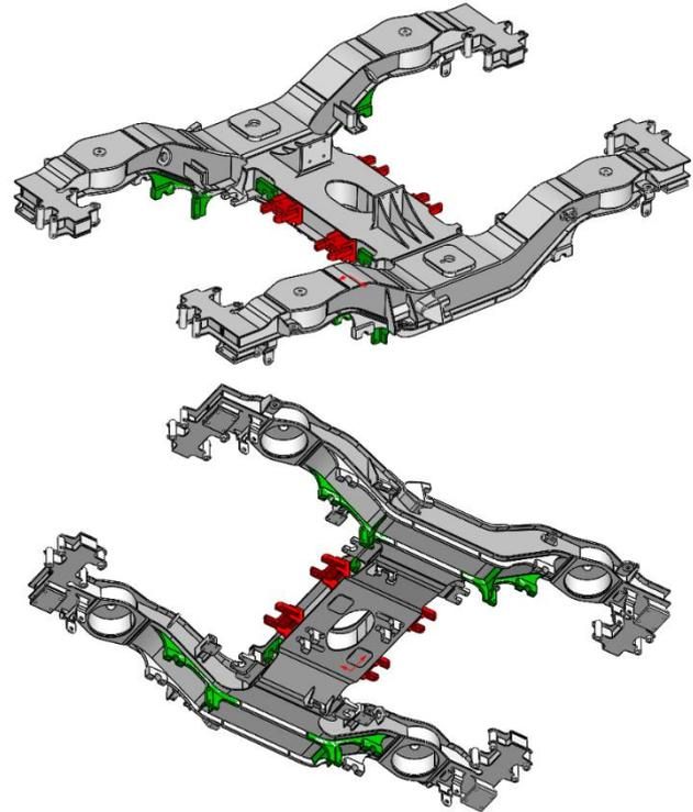
Fig. 3. Complete bogie frame with brackets
