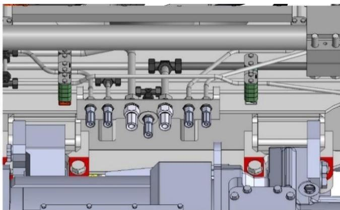
were screwed to the profiles using system T-nuts, allowing the clamps to move freely along the length of the profile. Pneumatic installation – just like the electric one, it has its connection in the central part of the bogie.
