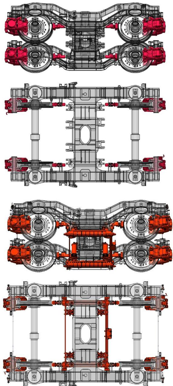
Fig. 10. Braking system of the 41MN type bogie (above) and the 46AN type bogie (below)
