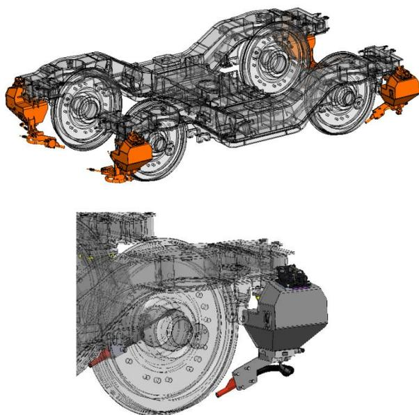
Fig. 14. Sanding system of the 41MN driving bogie
