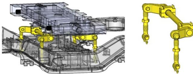
Fig. 11. Body anti-roll bar
