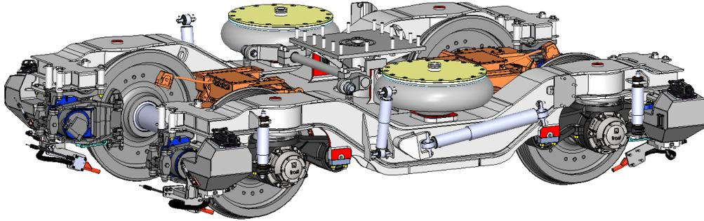
Fig. 1. Driving bogie type 41MN
