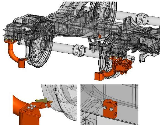
Fig. 13. Flange lubrication system of the 46AN bogie
