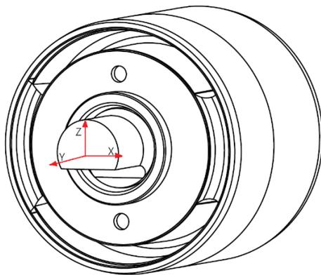
Fig. 5. Isometric view of a rubber-metal joint
