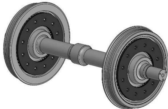
Fig. 4. Isometric view of the wheelset of the motor bogie
