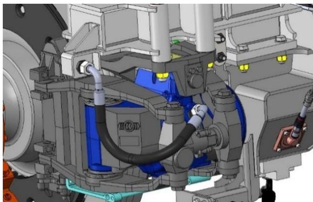
Fig. 16. The system of pneumatic hoses on the 41MN bogie
