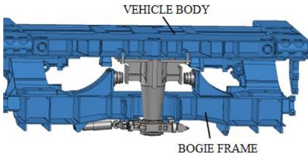
Fig. 9. System of transmission of tractive force in bogies type 41MN and 46AN
