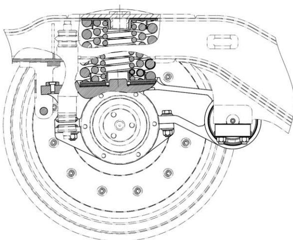
Fig. 6. Primary suspension of 41MN and 46AN bogies
