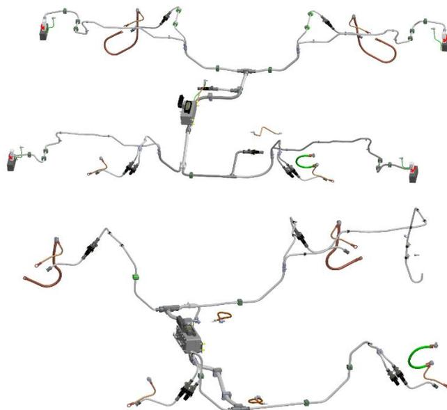
Fig. 15. Electric wiring for the 41MN (above) and 46AN (below) bogies
