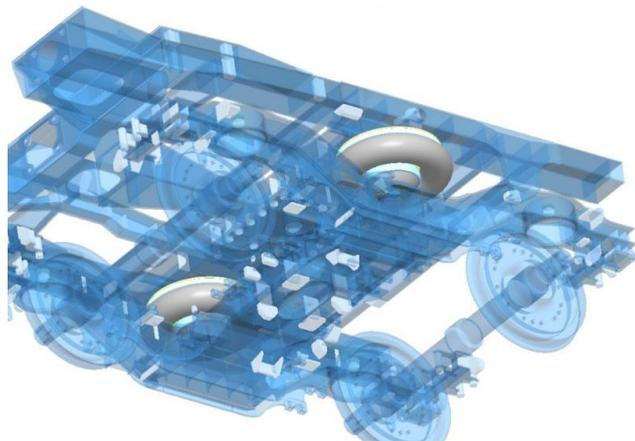
Fig. 7. Secondary suspension assembly for 41MN and 46AN bogies
