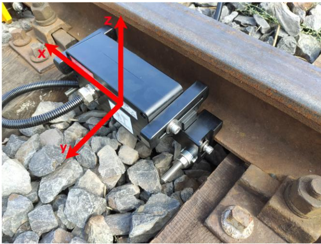
Fig. 1. Rail-mounted measuring antenna with the indicated directions of the plane
