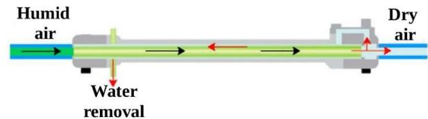
Fig. 3. Operational principle of a membrane dryer [1]
