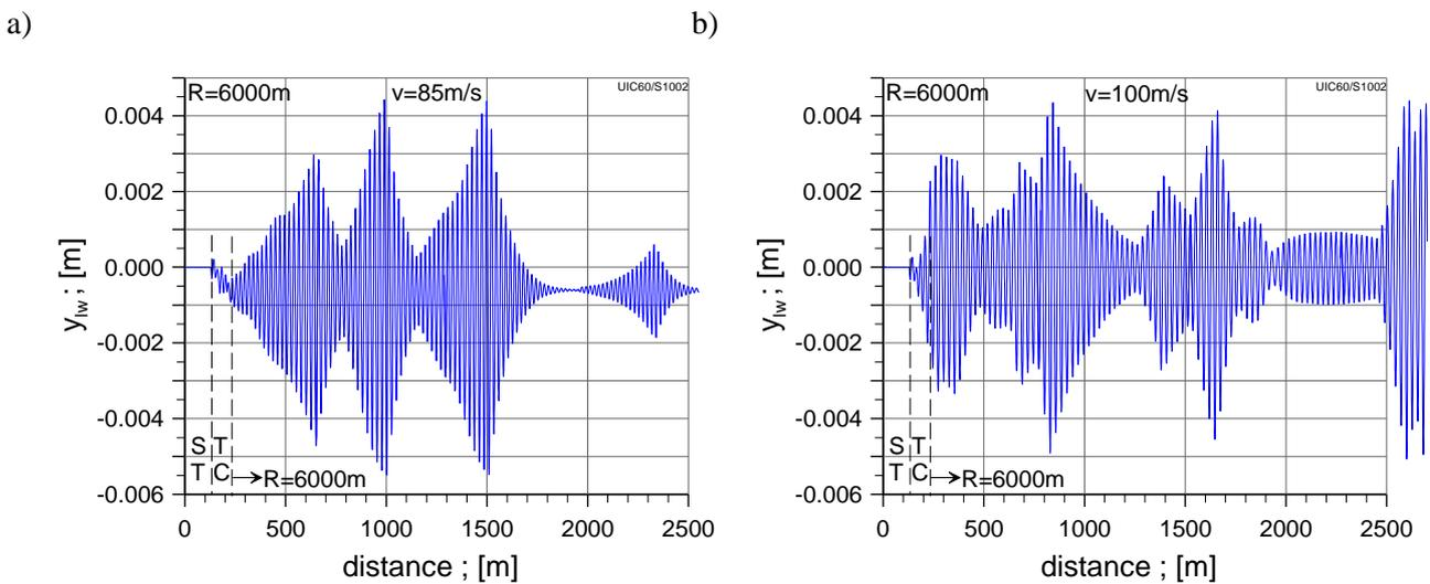
Fig. 8. The leading wheelset lateral displacements  $y_{lw}$  versus distance consist of: straight track section (ST), transition curve (TC) and regular arc  $R = 6000$  m. Vehicle velocity  $v$ : a)  $85$  m/s, b)  $100$  m/s, c)  $130$  and d)  $145$  m/s
