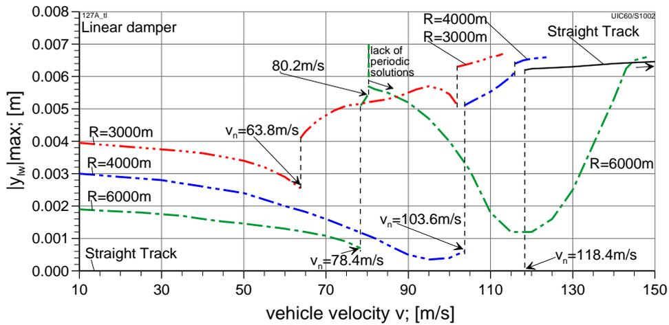
Fig. 7. Maximum of the leading wheelset lateral displacements absolute value versus vehicle velocity in straight track and curved track of curve radius  $R = 3000, 4000$  and  $6000$  m. Linear a-y dampers (ld) applied
