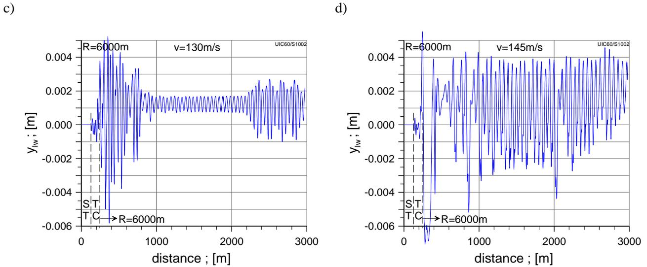
Fig. 8cd. The leading wheelset lateral displacements  $y_{lw}$  versus distance consist of: straight track section (ST), transition curve (TC) and regular arc  $R = 6000$  m. Vehicle velocity  $v$ : a) 85 m/s, b) 100 m/s, c) 130 and d) 145 m/s
