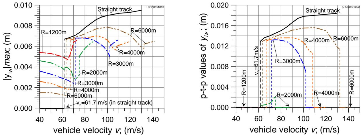
Fig. 5. Maximum of leading wheelset lateral displacements absolute value ( $|y_{lw}|_{max}$ ) and peak-to-peak values of  $y_{lw}$  versus vehicle velocity. Model without the anti-yaw dampers
