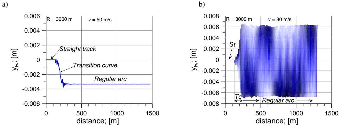
Fig. 4. The first wheelset lateral displacements  $y_{lw}$  versus distance: a) stable stationary solutions ( $50 \text{ m/s} < v_n$ ), b) stable periodic solutions (limit cycle,  $80 \text{ m/s} > v_n$ )
