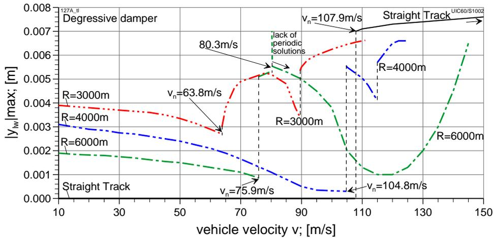
Fig. 6. Maximum of the leading wheelset lateral displacements absolute value versus vehicle velocity in straight track and curved track of curve radius  $R = 3000, 4000$  and  $6000$  m. Degressive a-y dampers (dd) applied
