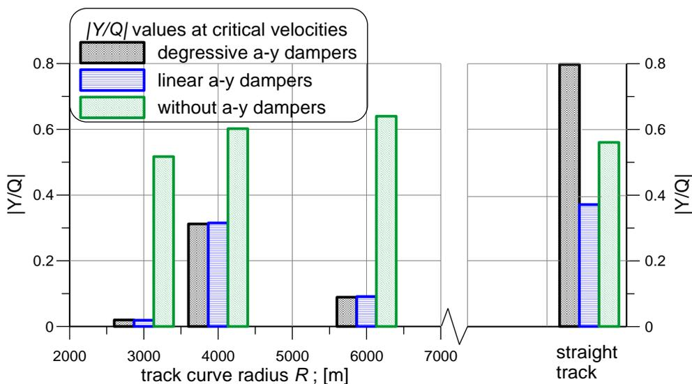
Fig. 13. Comparison of a-y dampers influence on derailment ratio (|Y/Q|) at critical velocities v<sub>n</sub> (collected in Table 2) in straight track and curved track of curve radius R = 3000, 4000 and 6000 m
