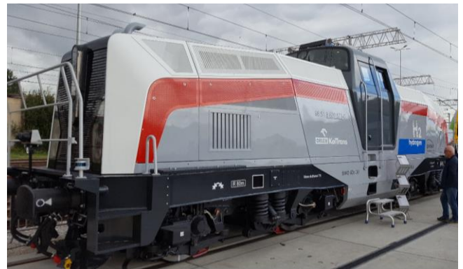
Fig. 2. The SM42 6Dn hydrogen shunting locomotive presented by PESA at the TRAKO rail fair
