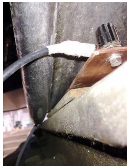
Fig. 5. Placement of the measuring probe
