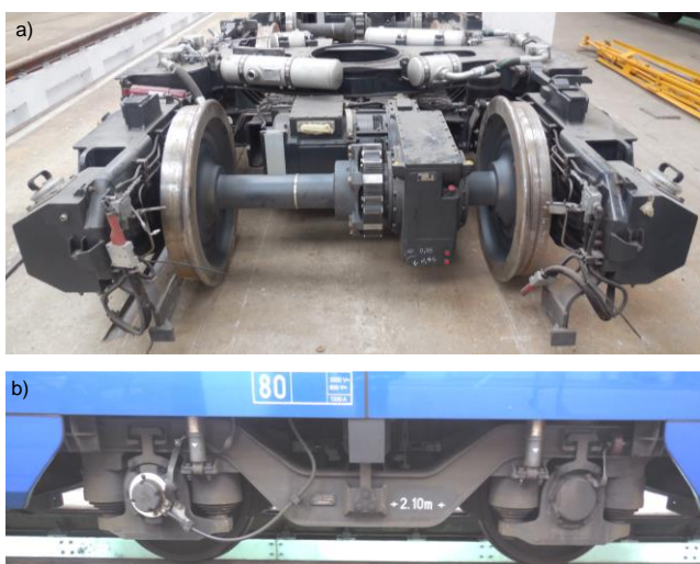
Fig. 3. View of the bogies of the EN97 vehicle: a) the 34MN driving bogie disassembled with the transmission and traction motor visible, b) the view of the 4AN rolling bogie under the middle section
