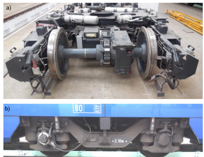
Fig. 3. View of the bogies of the EN97 vehicle: a) the 34MN driving bogie disassembled with the transmission and traction motor visible, b) the view of the 4AN rolling bogie under the middle section
