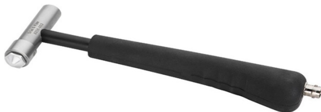
Fig. 8. Brüel & Kjær type 8206 modal hammer - manufacturer's diagram [3]
