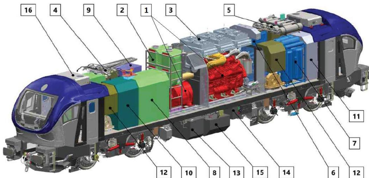
Fig. 4. Layout of equipment on the 111DE locomotive, 1 – power generator, 2 – a set of SCR catalytic systems, 3 – combustion engine cooling unit, 4 – pantograph, 5 – main air tanks, 6 – compressor module, 7 – board module, 8 – power inverters cabinet, 9 – cooling column with braking resistor, 10 – HV cabinet, 11 – ETCS cabinet, 12 – LV cabinet with electric motors ventilator, 13 – line choke, 14 – battery box, 15 – fuel tank, 16 – air conditioning unit [19]
