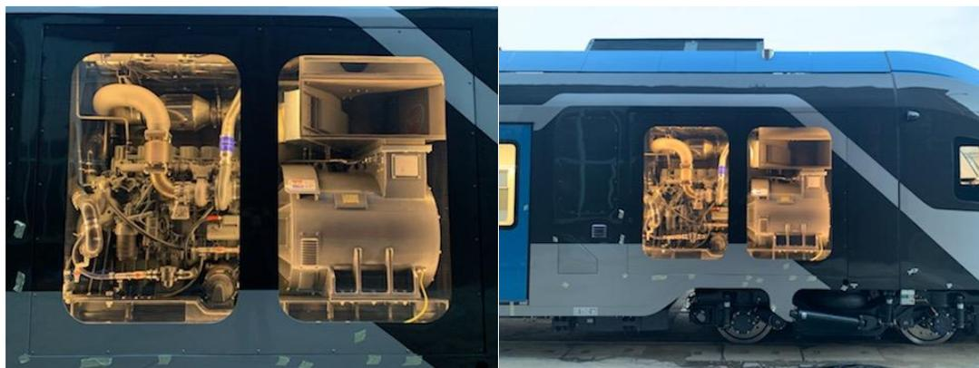
Fig. 3. Built-in powerpack generator in the type 227M rail vehicle [8]
