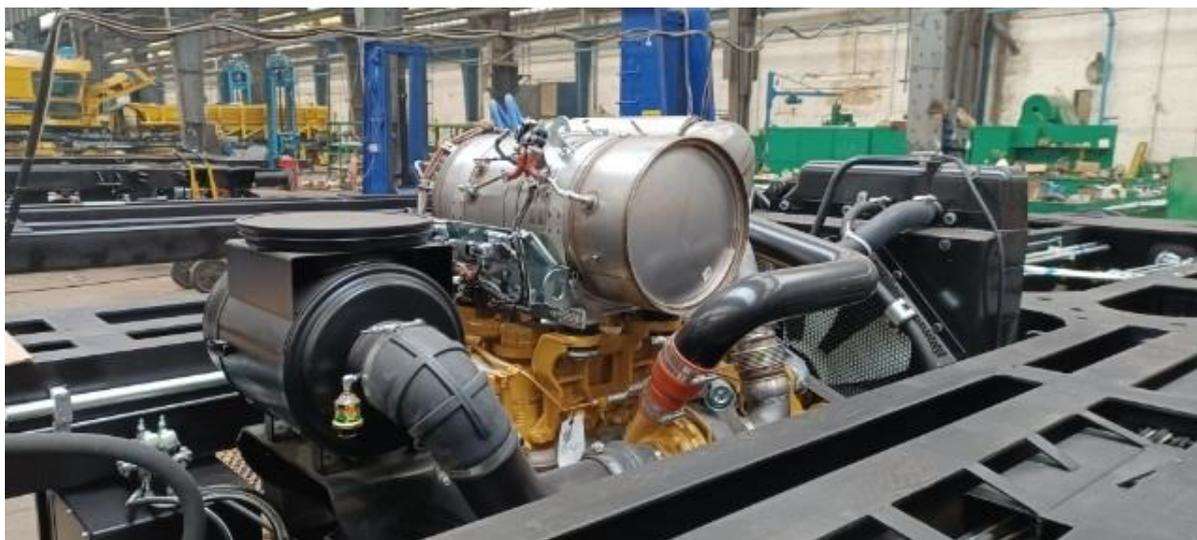
Fig. 12. An example of a CAT engine mounted in the free undercarriage space of a different type special purpose rail vehicle
