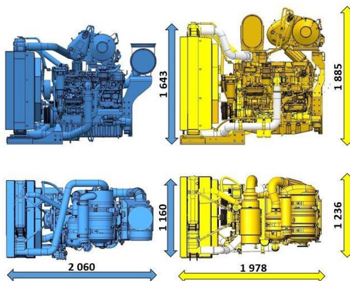
Fig. 11. List of internal combustion engines proposed for installation on the 501EH vehicle with dimensions provided. Top image shows the side view, bottom image shows the top view. Blue color CAT C9.3B engine, yellow color CAT C13B
