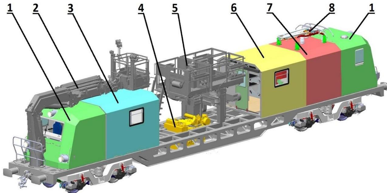
Fig. 9. The initial concept schematic of a 501EH special purpose vehicle; 1 – driver's cabin, 2 – cherry picker basket and arm, 3 – crew rest compartment, 4 – combustion engine, 5 – cherry picker platform, 6 – workshop compartment, 7 – electrical module, 8 – pantograph
