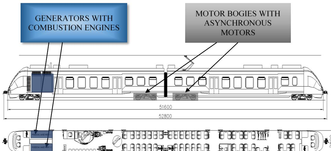
Fig. 2. Location of generating sets and motor bogies [8]
