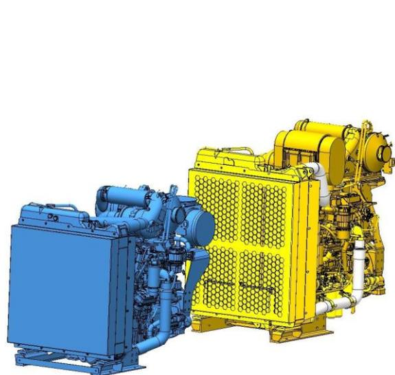
Fig. 10. A list of internal combustion engines proposed for installation on the 501EH vehicle. Blue color CAT C9.3B engine, yellow color CAT C13B
