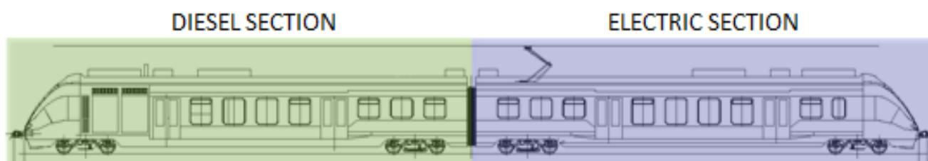
Fig. 1. Type 227M rail vehicle consisting of two segments: diesel and electric [28]
