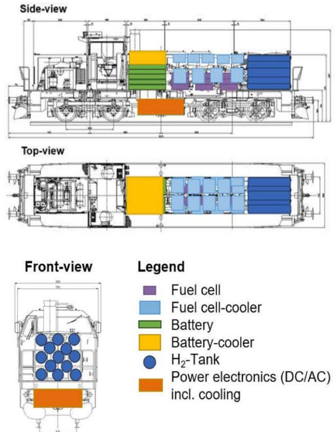
Fig. 8. Arrangement of the components on a MaK G1206 locomotive [15]
