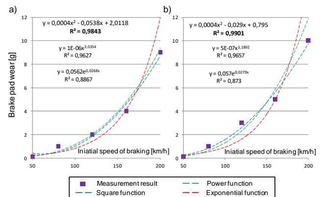
Fig. 4. The relationship of brake pad wear as a function of initial speed at  $N = 28$  kN and  $M_h = 6.7$  t, braking with: a) new 35 mm brake pads, b) 15 mm brake pads
