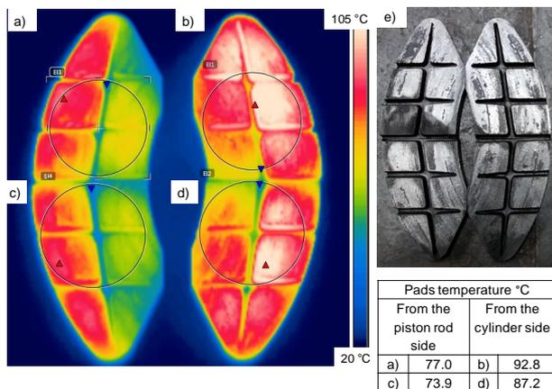
Fig. 6. Temperature distribution on the brake pads, a) upper left pad, b) upper right pad, c) lower left pad, d) lower right pad, e) View of the set of brake pads after braking from the speed of 120 km/h
