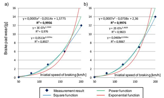
Fig. 3. The relationship of brake pad wear as a function of initial speed at  $N = 40$  kN and  $M_h = 6.7$  t, braking with: a) new 35 mm brake pads, b) 15 mm brake pads
