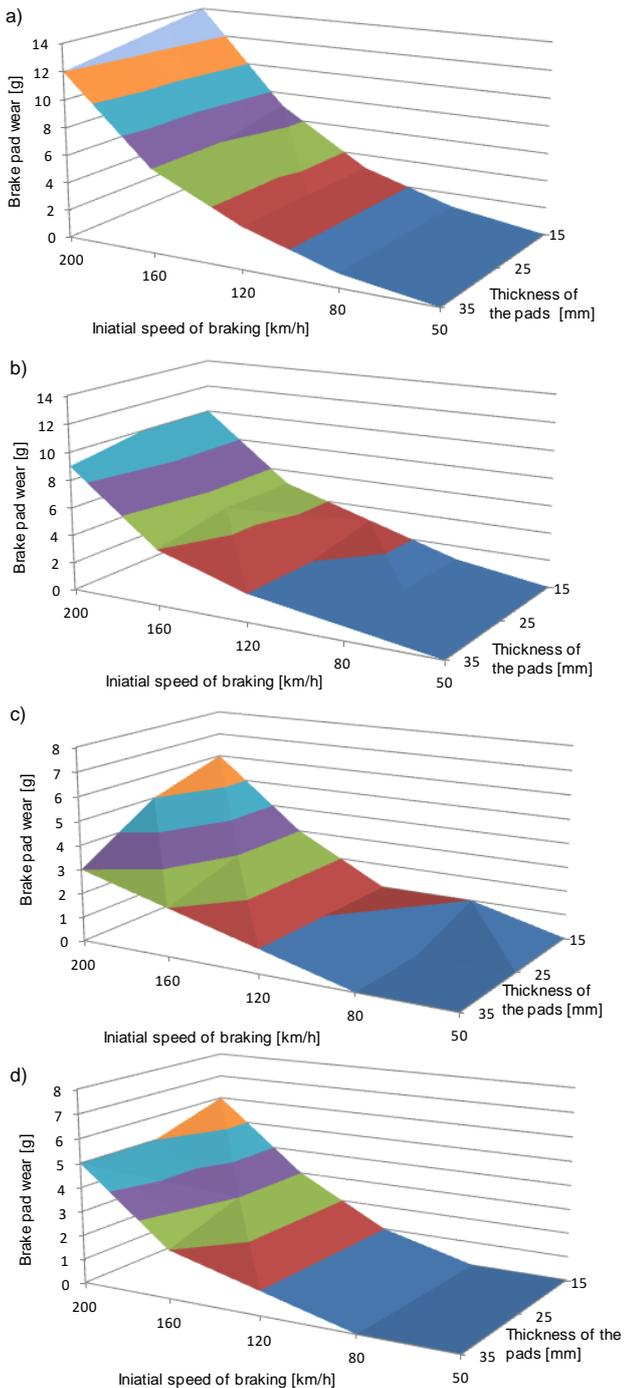
Fig. 5. Mass wear of the pads at: a)  $N = 40$  kN,  $M_h = 6.7$  t, b)  $N = 28$  kN,  $M_h = 6.7$  t, c)  $N = 26$  kN,  $M_h = 4.7$  t, d)  $N = 16$  kN,  $M_h = 4.7$  t
