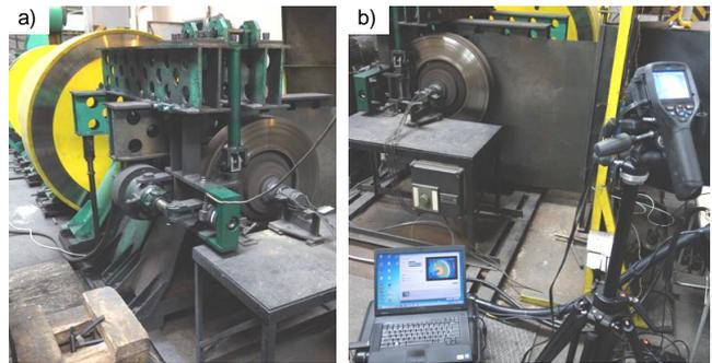
Fig. 1. Stand for testing a railway disc brake: a) view of the working part with rotating masses, b) view of the tested brake disc with thermal imaging measurement
