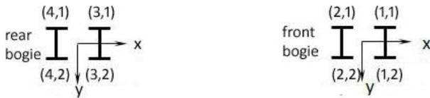
Fig. 6. Identification of wheel positions in a four-axle metro car model
