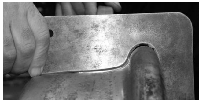
Fig. 4. Visualisation of wear on the wheel running surface [8]
