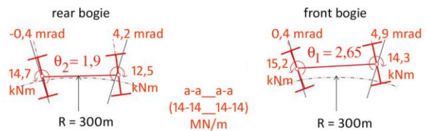
Fig. 17. Position of bogies of a metro car model with a symmetrical 14 – 14__14 – 14 configuration of wheelset guidance stiffness on a full curve of track with a radius of 300 m
