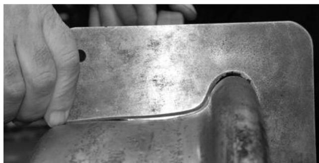
Fig. 4. Visualisation of wear on the wheel running surface [8]
