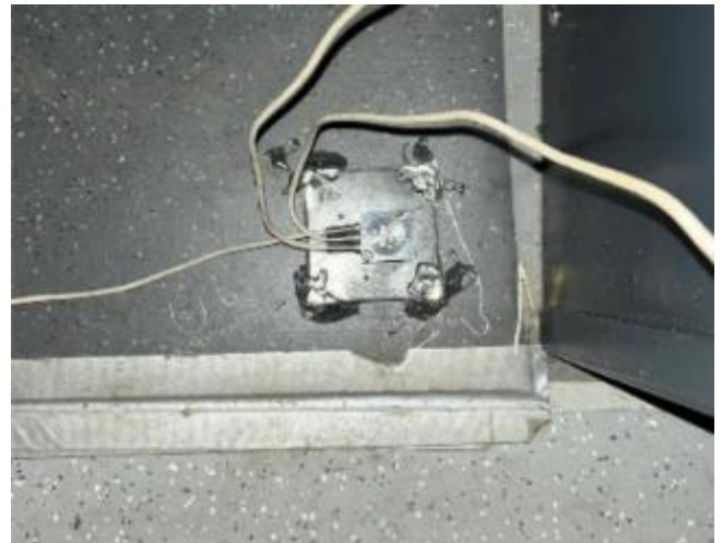
Fig. 10. Measurement point 2 localized on the train floor
