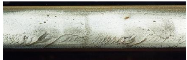
Fig. 2. Example of a "head checks" defect [15]
