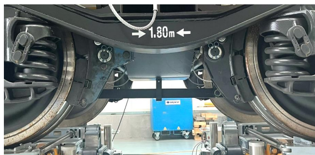
Fig. 2. Freight wagon with a block brake on a test bench
