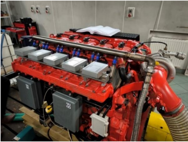
Fig. 4. The test stand with an internal combustion engine adapted to run on hydrogen at the Krakow University of Technology [2]
