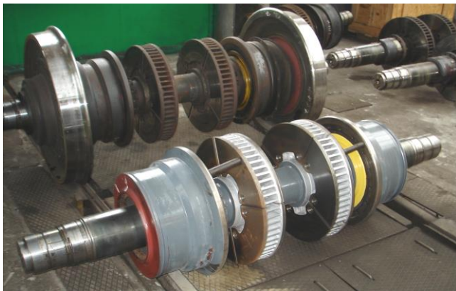
Fig. 15. View of the axle and the 1435/1520 mm SUW 2000 adjustable wheel set with split discs [W. Sawczuk]
